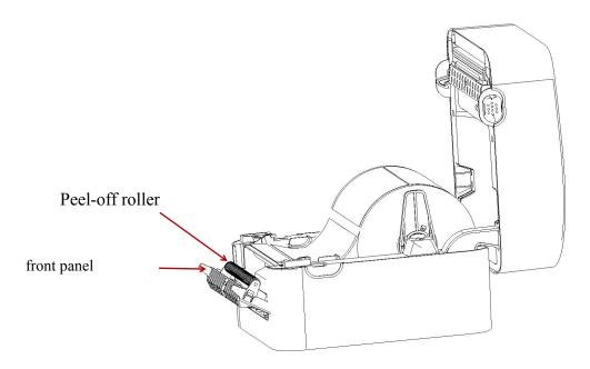
2. Pass the label through the paper guide, and pull the label over the rubber roller.
