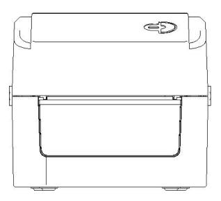
Note: To avoid poor printing quality, make sure the printer cover is closed tightly.
